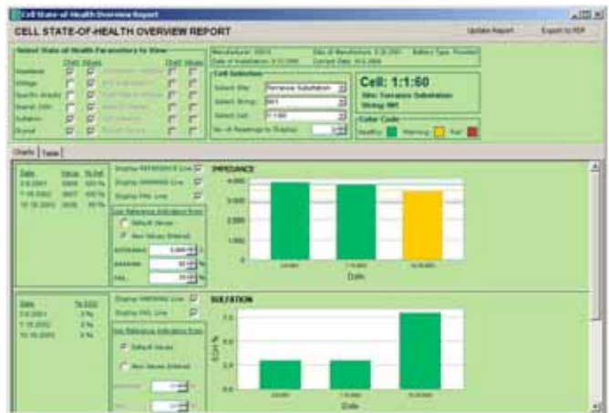
The cell level report window - accessible directly from the inventory overview or the string level report - provides the user with trended profiles for any of the recorded test data for any cell or monoblock
