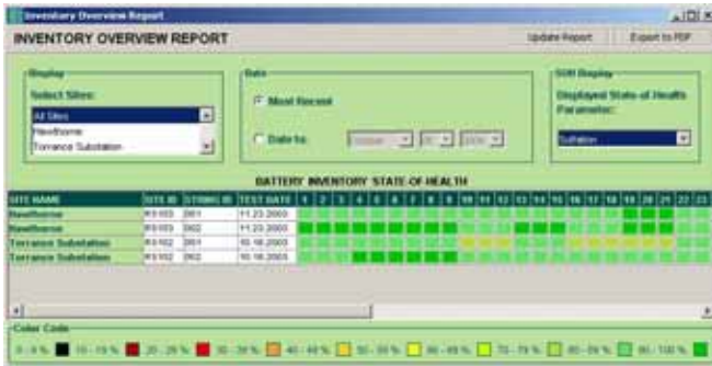
The Inventory Overview screen allows the user an "at-a-glance" view of the state of health of the entire battery inventory
